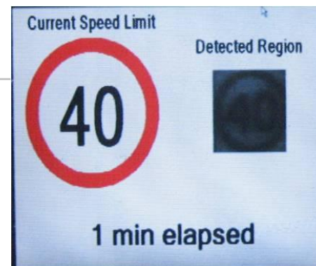
Speed sign recognition system – in car display showing the driver the prevailing speed limit and time since passing last sign
