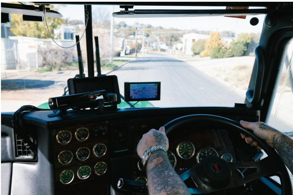
*Eye and face tracking software can detect driver distraction, and provide context in the event that a collision cannot be avoided*
