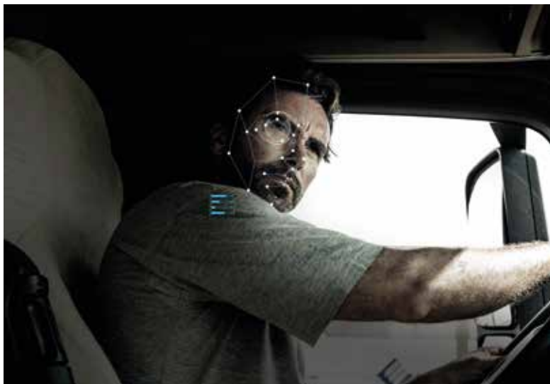
Eyes straight ahead: Seeing Machines' Guardian camera tracks head movements
